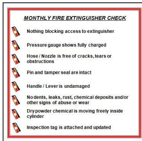
Figure 17: tasks for monthly maintenance of an extinguisher
