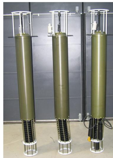
Figure 2: Three SWARM floats, ready for testing
